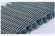
Mar-Con Square Weave is assembled with flat connector strips instead of the crimped wires normally used. The flat strips allow the use of a spiral that forms a nearly perfectly flat surface. This allows the removal of products that may have a tendency to stick. Additionally, the load of the product is more evenly distributed, reducing the possibility of marking on soft products.
