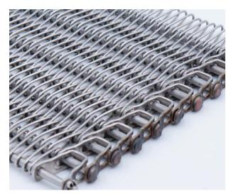
Mar-Con Spiral Freezer Belting is designed to be used in applications where the conveyor belt must travel in a curved rather than a straight path. It consists of a series of cross connector rods with special collapsible chain links along each edge.
