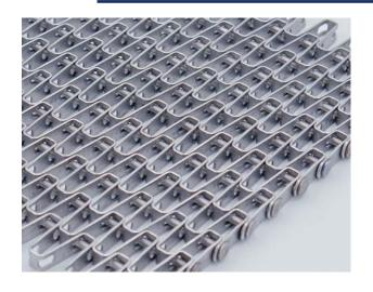
Mar-Con Flat Wire Belt is an inexpensive, yet rugged style of conveyor belt. It consists of a series of flat strips, bent into a zig-zag shape, and held together with a cross-connector wire.
