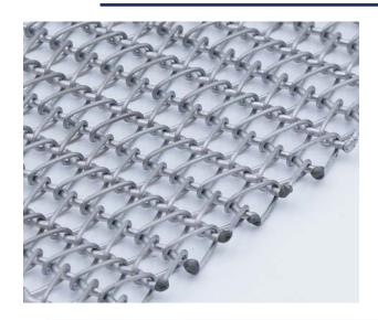
Equalized Weave is the most common style of conveyor mesh used. It consists of alternating Right-hand and Left-hand spirals joined together with either a crimped or straight connector wire.
