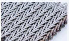
Mar-Con Baking Band is used in applications that require an extremely flat surface and very little open area. It consists of standard Equalized style spirals interwoven so that 3 or 4 spirals overlap. Baking Band style mesh is commonly found on cookie and cracker baking ovens, fried pie lines, tortilla bakers, glass lehrs, can accumulators and many other applications.
