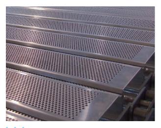
The Mar-Con Plateveyor is a special conveyor system made up of sheet metal plates and standard conveyor chain. It is one of the strongest and flattest conveyor available.
